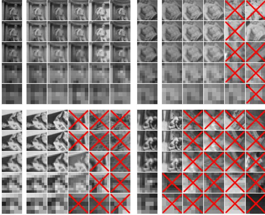
Figure 5: Examples of querying the Trevi Fountain patch dataset using different patch sizes. The query patch is on the left of each panel, while the following 5 patches are the nearest neighbors from a set of 100,000 patches. Incorrect matches are shown with an X.
